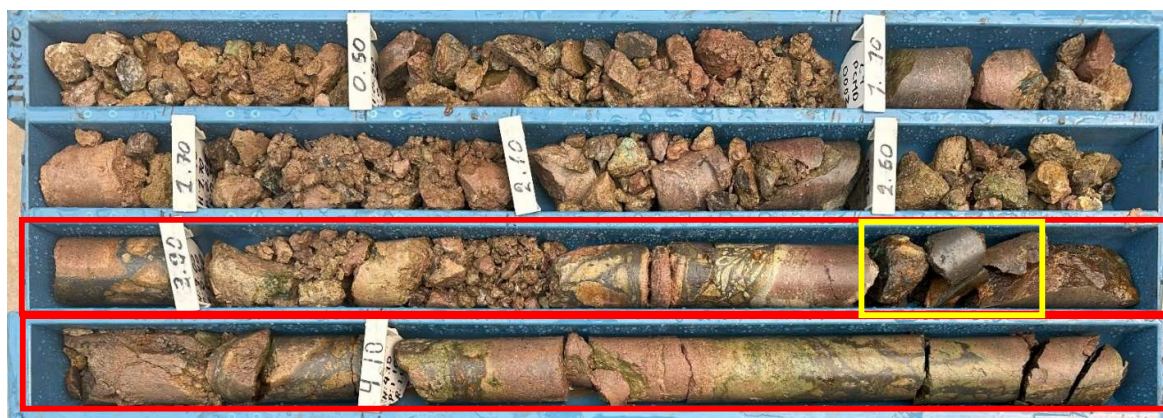
FIGURE 2: PICHA PROJECT – HIGH-GRADE COPPER-SILVER MINERALISATION AT COBREMANI TARGET (24PCMD0003 – 5.12M @ 5.4% CU AND 44.9G/T AG FROM 2.88M)
