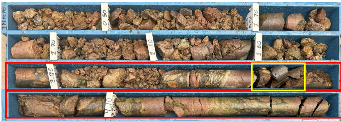
FIGURE 2: PICHA PROJECT – HIGH-GRADE COPPER-SILVER MINERALISATION AT COBREMANI TARGET (24PCMD0003 – 5.12M @ 5.4% CU AND 44.9G/T AG FROM 2.88M)
