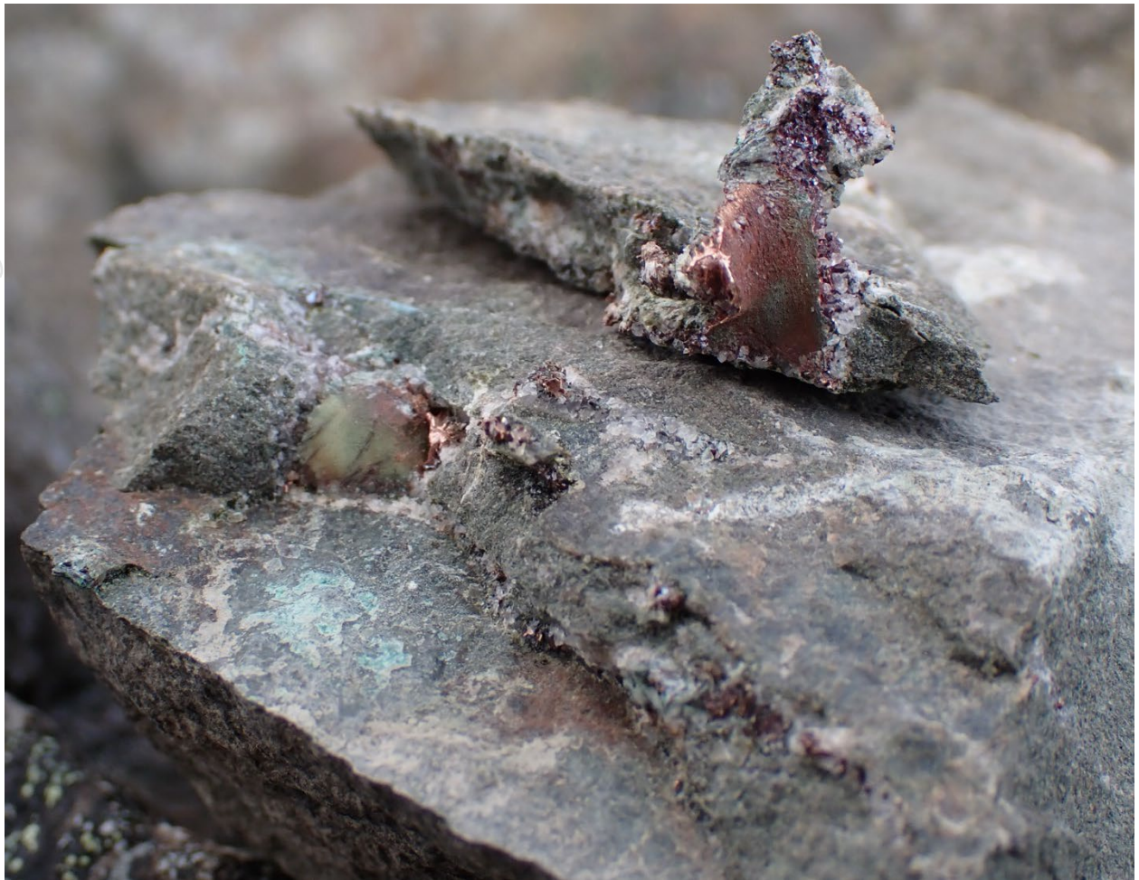
Figure 8 - Example of native copper mineralisation from the southern extent of the HALO vein system. Field of view 10 cm. (Sample F005999).
