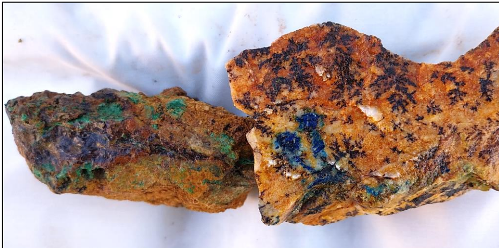
Figure 1. Sample PER015, recently collected near shallow unnamed workings at the southern end of the Black Ridge copper trend during reconnaissance mapping. The sample contains secondary copper carbonates (blue and green) in a fractured limestone host, with assays for the sample returning 6.5% Cu, 0.16g/t Au & 16g/t.
