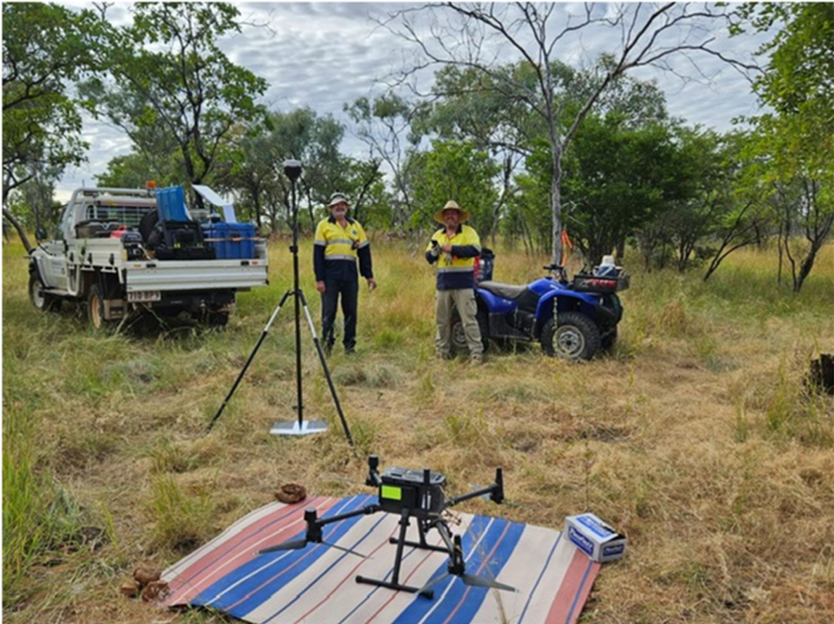
Figure 3. Drone LIDAR, Photogrammetry Survey station at Fiery Creek Copper Prospect
