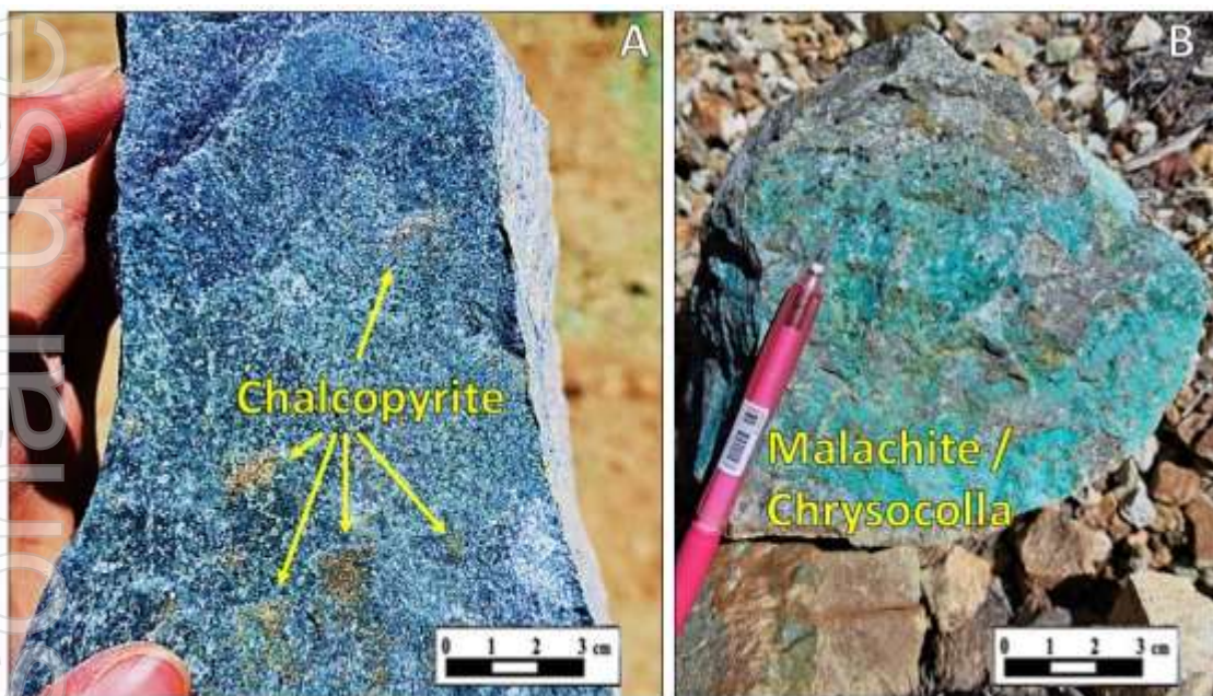
Example of mineralisation identified at the La Florida Prospect, A: Copper sulphide present as chalcopyrite Sample # CPO0008692 - 3.18% Cu and 2.61g/t Au, B: Copper oxide present as malachite and chrysocolla Sample #CPO0008688 - 3.96% Cu and 1.17g/t Au 1 .
