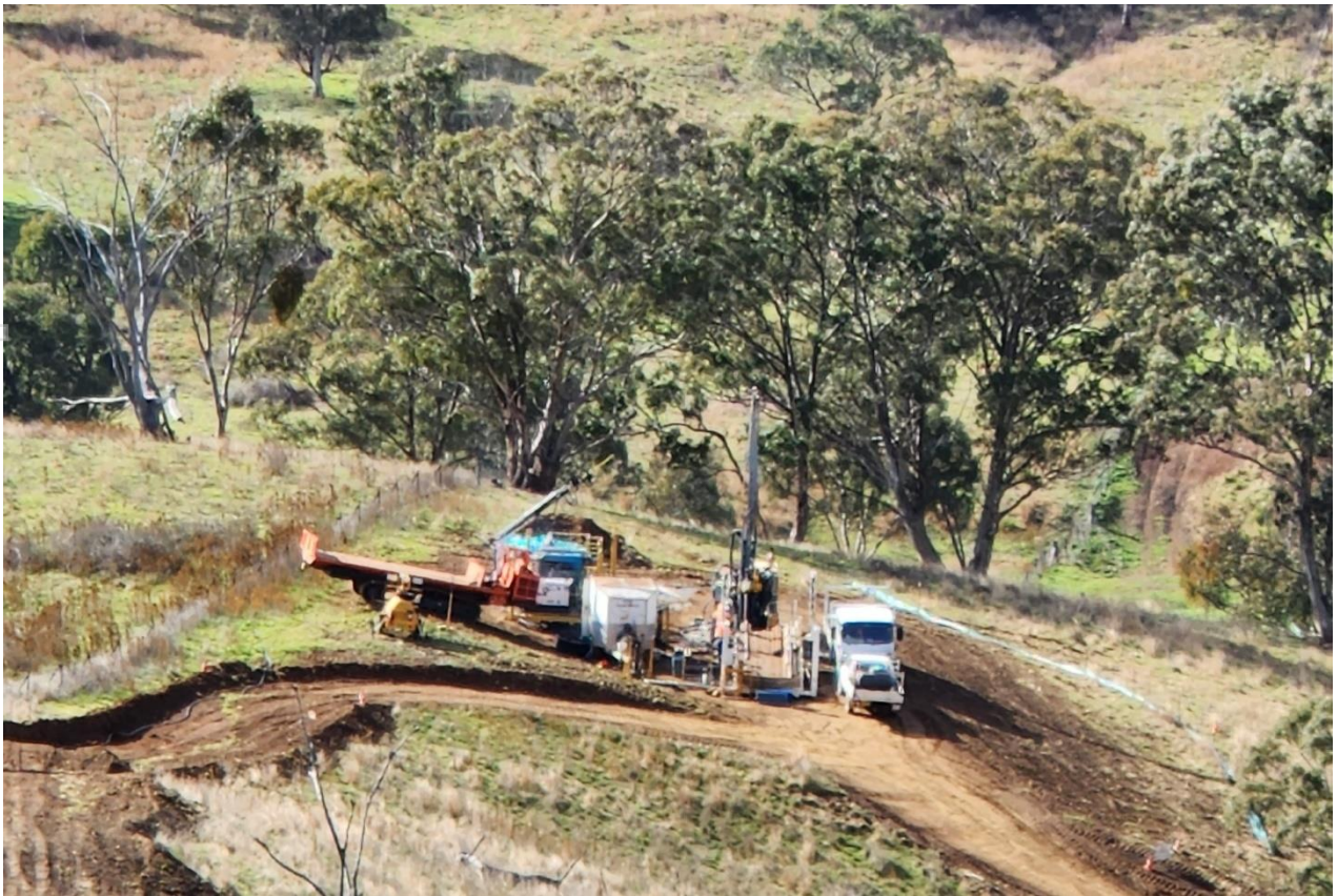
Image 1: Diamond drilling testing IP anomaly copper-gold-silver sulphide targets at Havilah Project, NSW
