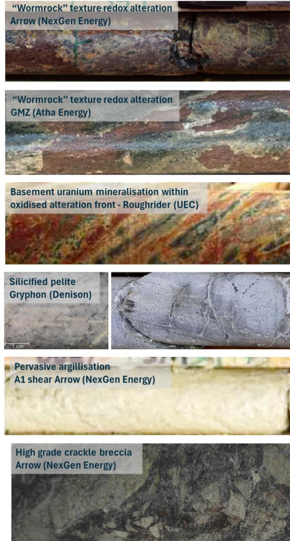
Figure 3 8 : Comparison of alteration styles encountered in drill core at Preston Creek (left photos) compared to mineralised basement-hosted alteration equivalent (right photos)
