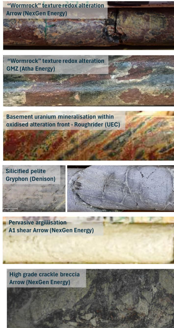
Figure 3 8 : Comparison of alteration styles encountered in drill core at Preston Creek (left photos) compared to mineralised basement-hosted alteration equivalent (right photos)
