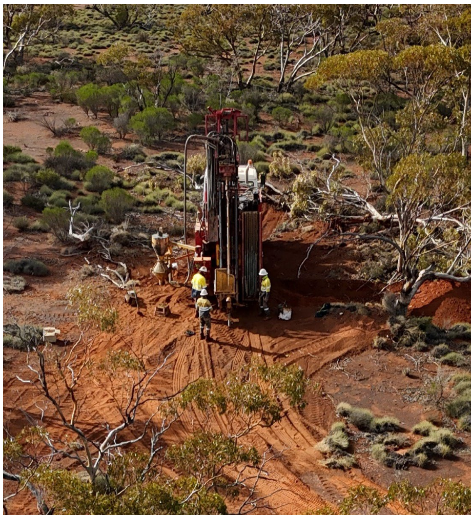
Image 2 – Slimline RC drill rig at Rogan Josh Prospect
