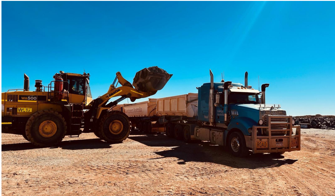
Figure 10- ROM Loader placing Second Fortune gold ore into road train (April 2024)
