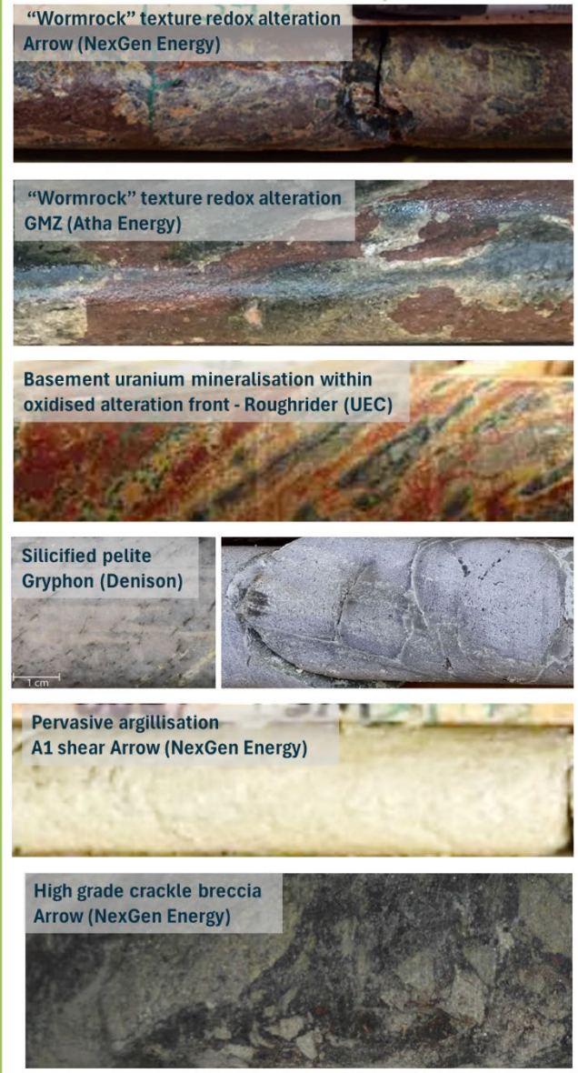
Figure 3: Comparison of alteration styles encountered in drill core at Preston Creek (left photos) compared to mineralised basement-hosted alteration equivalent (right photos)
