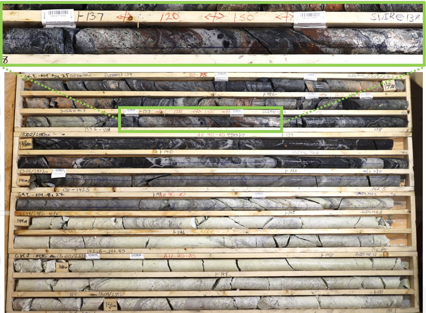
Figure 2: Core photograph of a radiometrically elevated altered breccia in drillhole GKI0014 which returned 190 ppm U_3O_8 .
