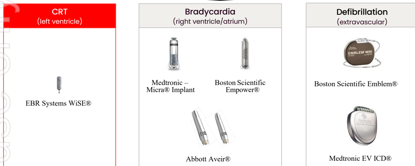
Figure 1.10: Current Leadless Pacemakers for Cardiac Pacing*
