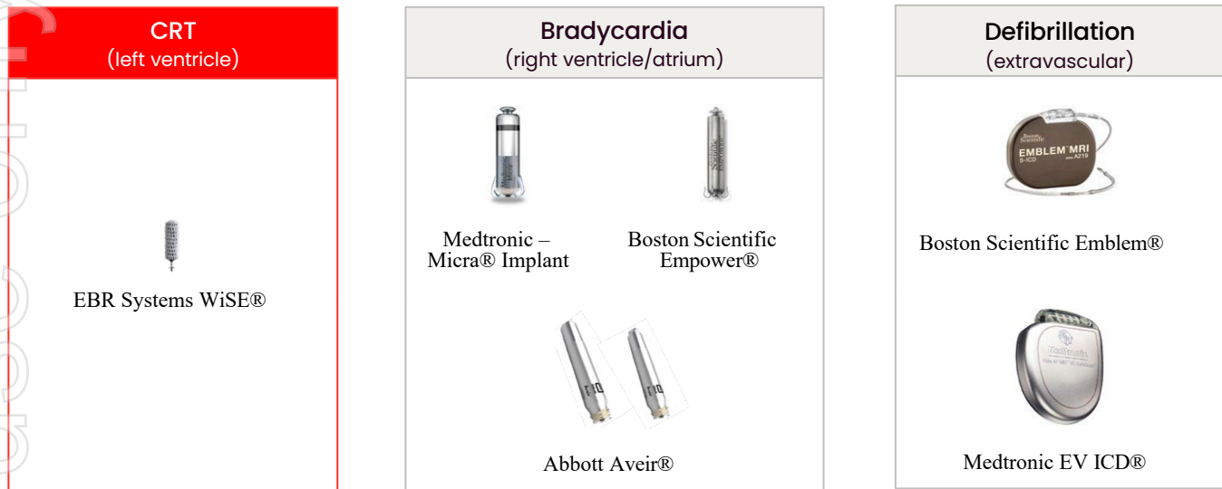
Figure 1.10: Current Leadless Pacemakers for Cardiac Pacing*
