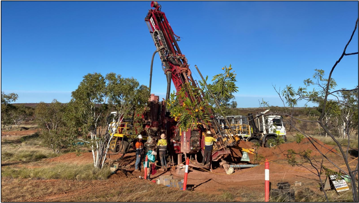
Image 1: Topdrill RC drilling rig testing for extensions of the Bluebird discovery
