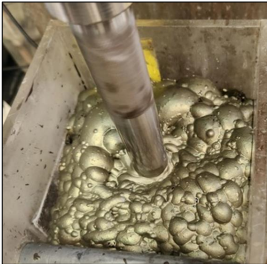
Image 2: Cleaner Flotation Concentration of Chalcopyrite from BBDD0045, Bluebird
