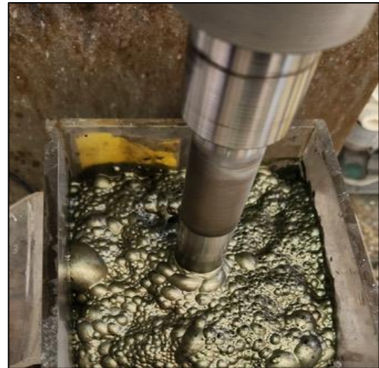
Image 2: Cleaner Flotation Concentration of Chalcopyrite from BBDD0045, Bluebird
