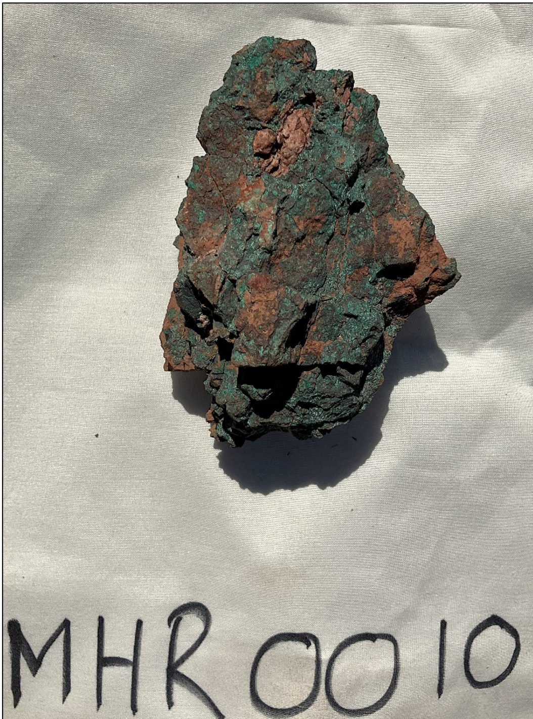
Photo 1: Sample MHR0010 which returned a grade of 45.5% Cu. Sample is ~7cm across. Sample location is shown in Figure 1.
