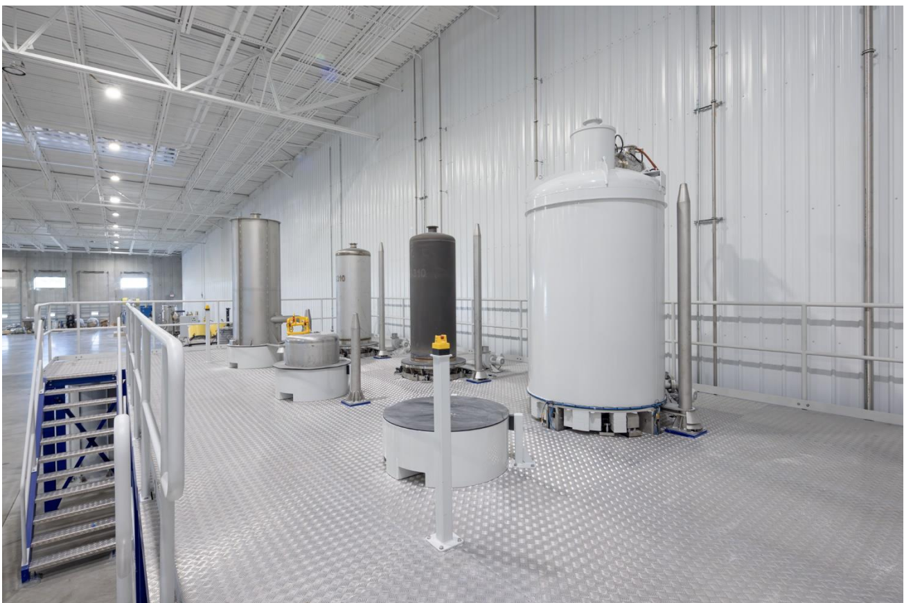
Figure 1: IperionX’s HAMR furnace deck, with site acceptance testing underway at the Titanium Production Facility
