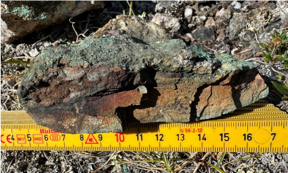
Figure 9 - Malachite along the bedding plane of and within a medium grained sandstone of the Rae Group sediments.
