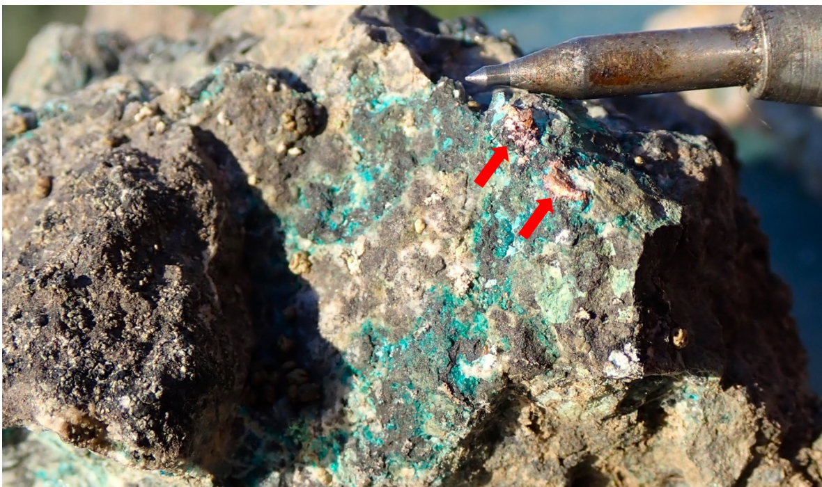
Figure 10 - Vesicular basalt flow top with chalcocite-malachite-chrysocolla-native copper mineralisation at the Kilauea target. Red arrows point to native copper within vesicles.
