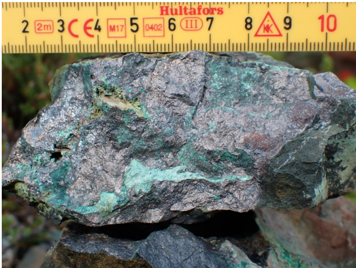
Figure 7 - Example of semi-massive bornite-chalcocite from the E/W trending DON vein system.
