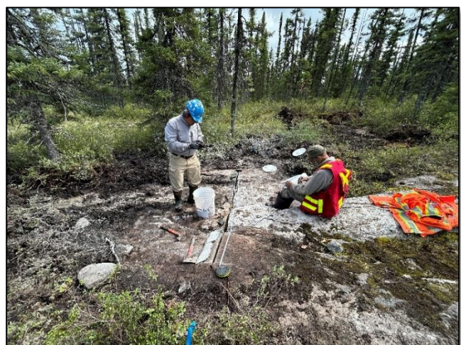
Photo 3 & 4: Western side of East Eade - Quartz outcrop exposed & diamond saw cutting & sampling. More program photos can be viewed on the company website.
