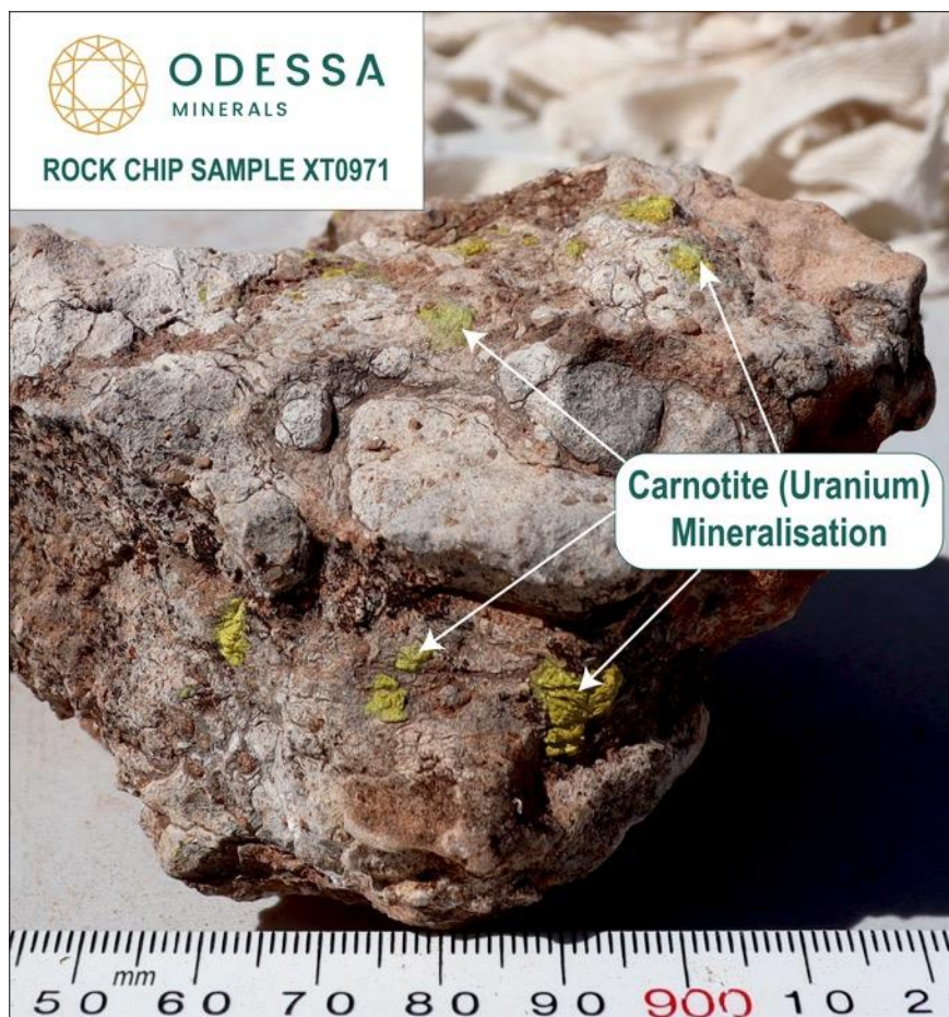
Figure 8: Carnotite (uranium) mineralisation within reworked siliceous calcrete at Baltic Bore in sample XT0971.
