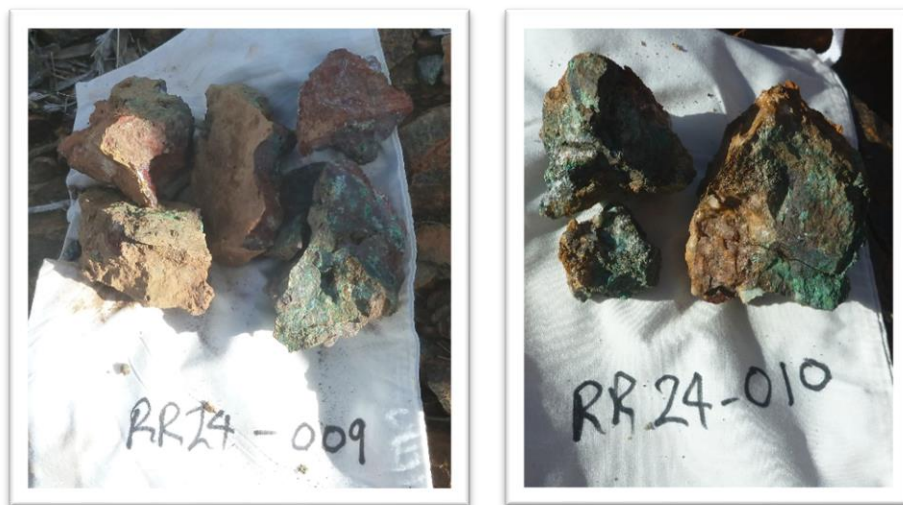
Figure 3. Rock chip samples RR24-009 (left) and RR24-010 (right) from the Scimitar Copper-Gold-Silver Prospect containing green malachite (copper) mineralisation.
