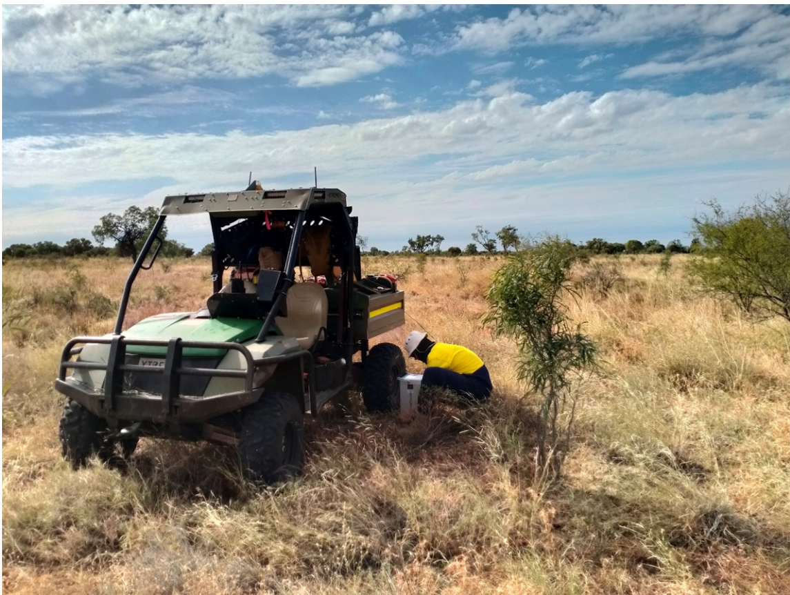
Figure 4: Daishat Geodetic crew conducting a gravity measurement at the Canobie FJV Project
