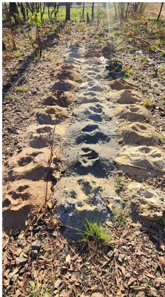
Figure 2: Aircore drill sample piles show distinct colour variation between host rocks (brown) and pegmatite/quartz veins (grey).
