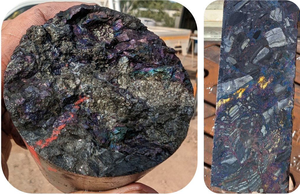
Examples of mineralisation in MOXD 217, 248.9-250m – 1.1m @ 24.8%Cu, 93.2 g/t Ag, 0.11% Co. Bornite, covellite, chalcocite and pyrite matrix fill hydrothermal breccia from within the broader intercept of 66.50m (48.00m estimated true width) @ 4.95% Cu, 32.7 g/t Ag and 685 ppm Co from 234.00m 5
