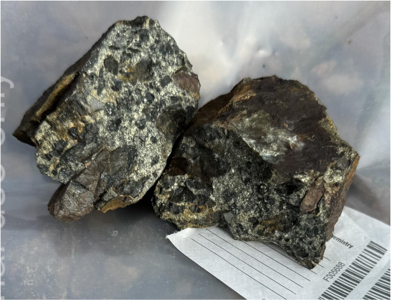
Figure 2 - Pyrite-chalcopyrite cemented breccia of phyllic altered andesite at the Cleaver IOCG target. (Sample F005688)
