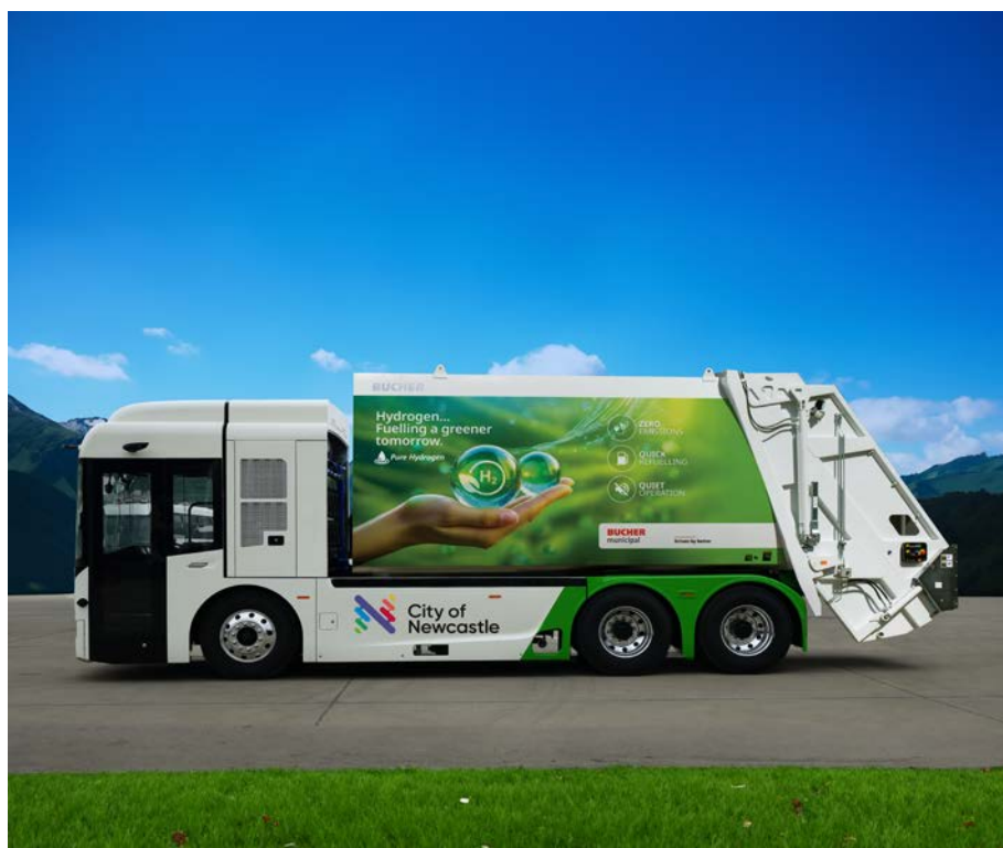
An image of the hydrogen fuel cell waste collection truck provided to City of Newcastle.
