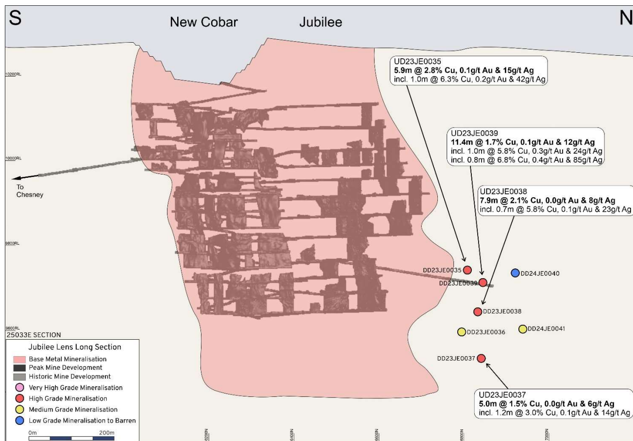
Figure 9: Long Section of the Jubilee deposit showing modern and historic development, the existing visible mineralisation envelope, and currently reported drillholes with significant intersections.
