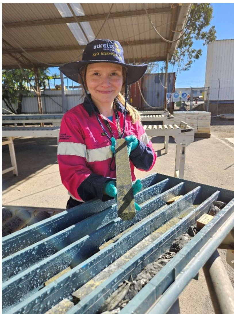
Figure 5: Exploration geologist Fernanda Alvarado-Neves holding drill core from Queen Bee drillhole DD24QB0041 from 440.4m to 440.75m, grading in-excess of 10% copper.
