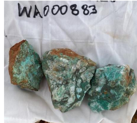
Copper rich brecciated quartz vein assayed 17.8% Cu, 65g/t Ag and 0.14g/t Au (Tiberius)
