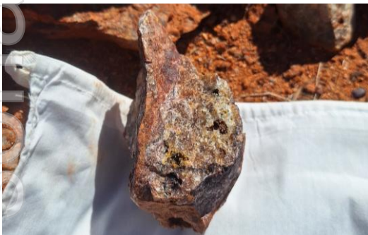
REE0012: 3.26g/t Au from gossanous quartz vein
