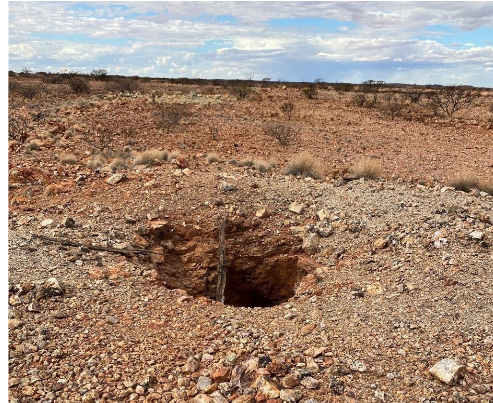
Prospecting shaft at Tiberius with extension of mineralised vein extending along the right of the picture.
