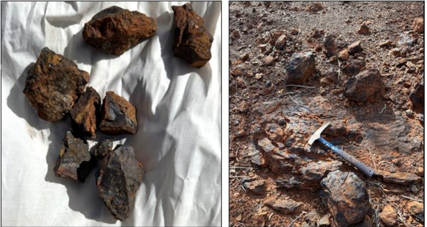
Figure 4: High grade rock chip BB7 60.63% Fe (left image), and area of enriched outcrop located 676,420mN and 7,150,310mN (right image).
