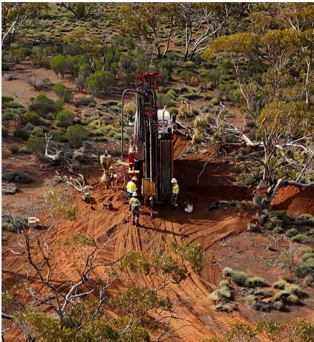
Image 1 – Slimline RC drill rig at Rogan Josh Prospect
