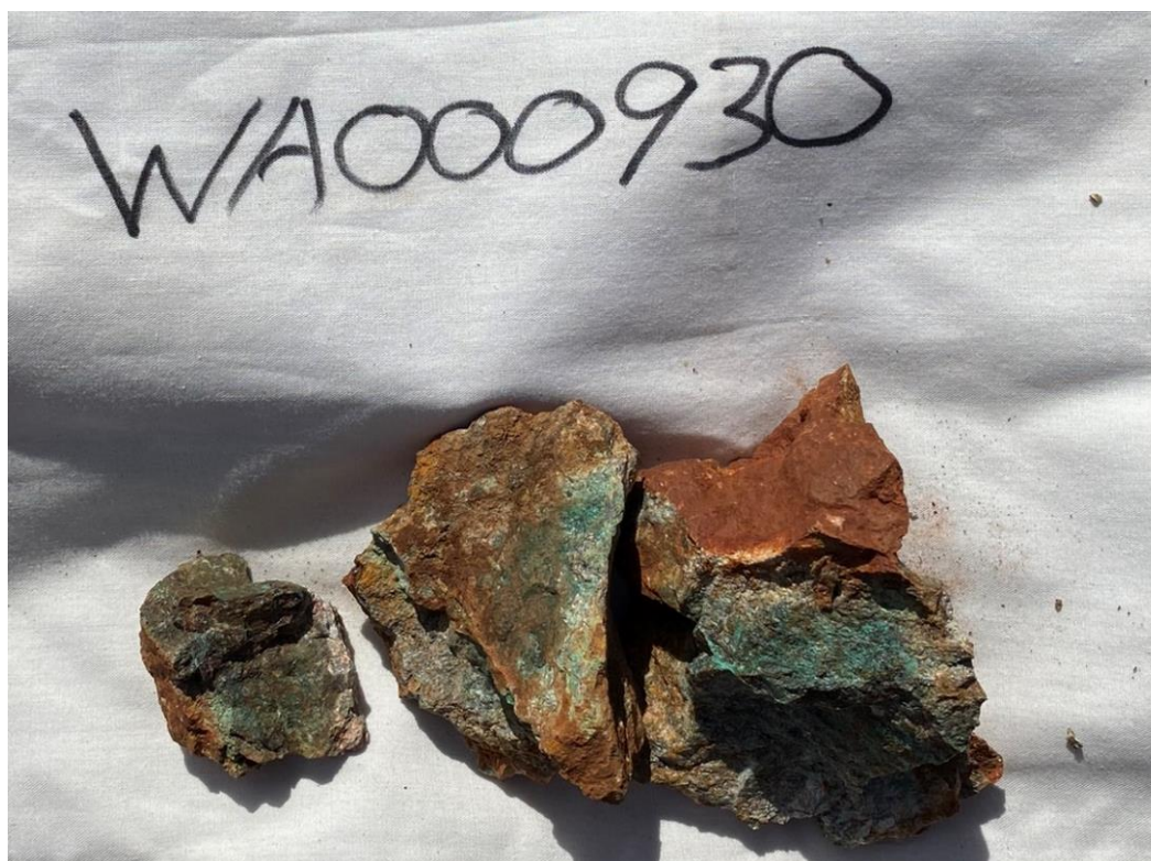
Figure 9 Quartz vein sample WA000930 which assayed 537ppm Mo.
