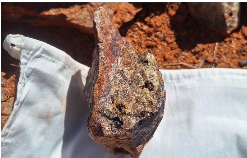
Figure 3 Sample REE0012 of gossanous quartz which assayed 3.26g/t Au at the South Snowy prospect.
