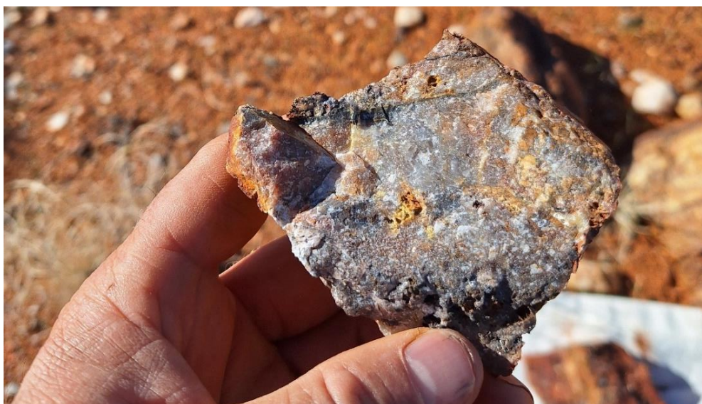
Figure 8 Quartz vein sample REE0071 which assayed 537ppm Mo.
