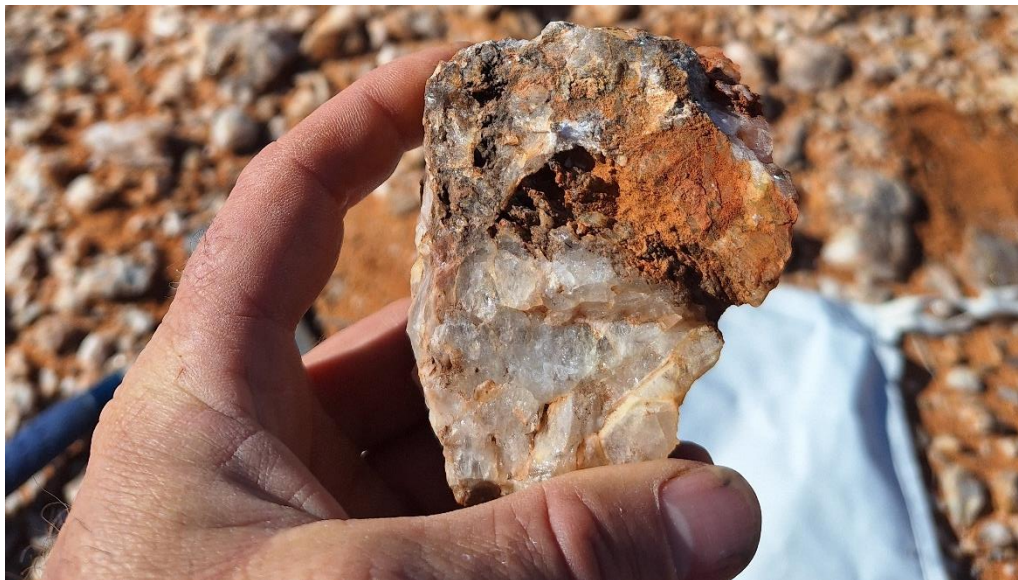
Figure 13 Sample REE0045 of vuggy vein quartz from the Peak Bore area which assayed 1,591ppm TREO.
