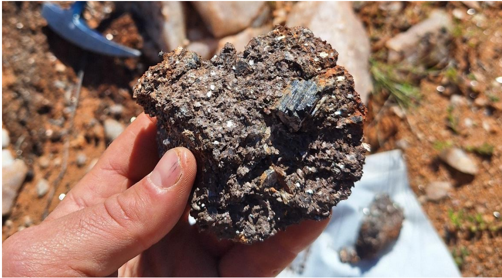
Figure 14 Sample REE0056 of muscovite and tourmaline rich pegmatite adjacent to a quartz vein from the Peak Bore area which assayed 1,591ppm TREO.
