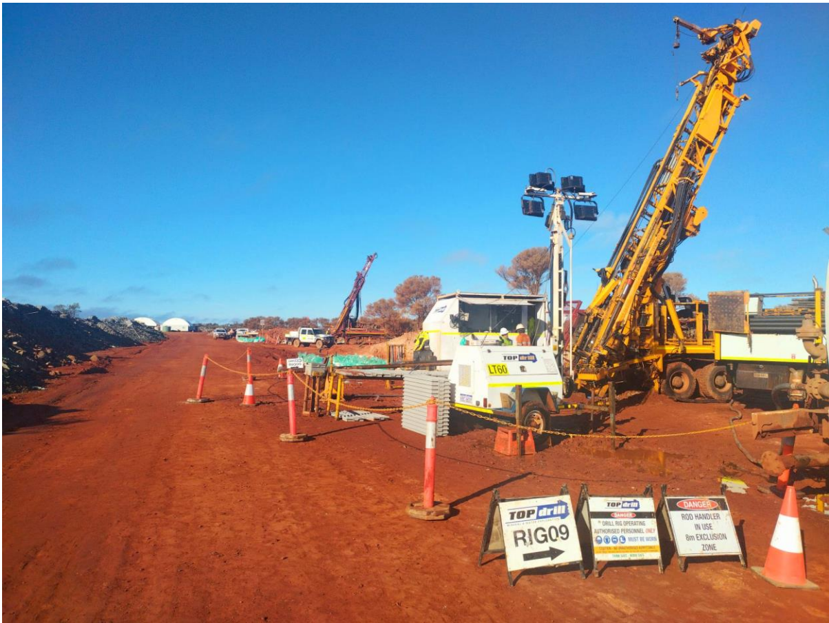
Figure 1 - Diamond (foreground) and RC (background) drill rigs at Second Fortune Gold Mine
