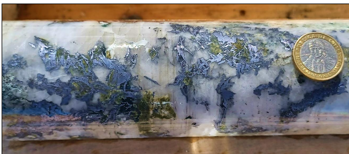
Figure 2: Example of high-grade molybdenum mineralisation in hole CMLCD014, 4,350ppm Mo ( 1.70\% CuEq) (498m to 500m).
