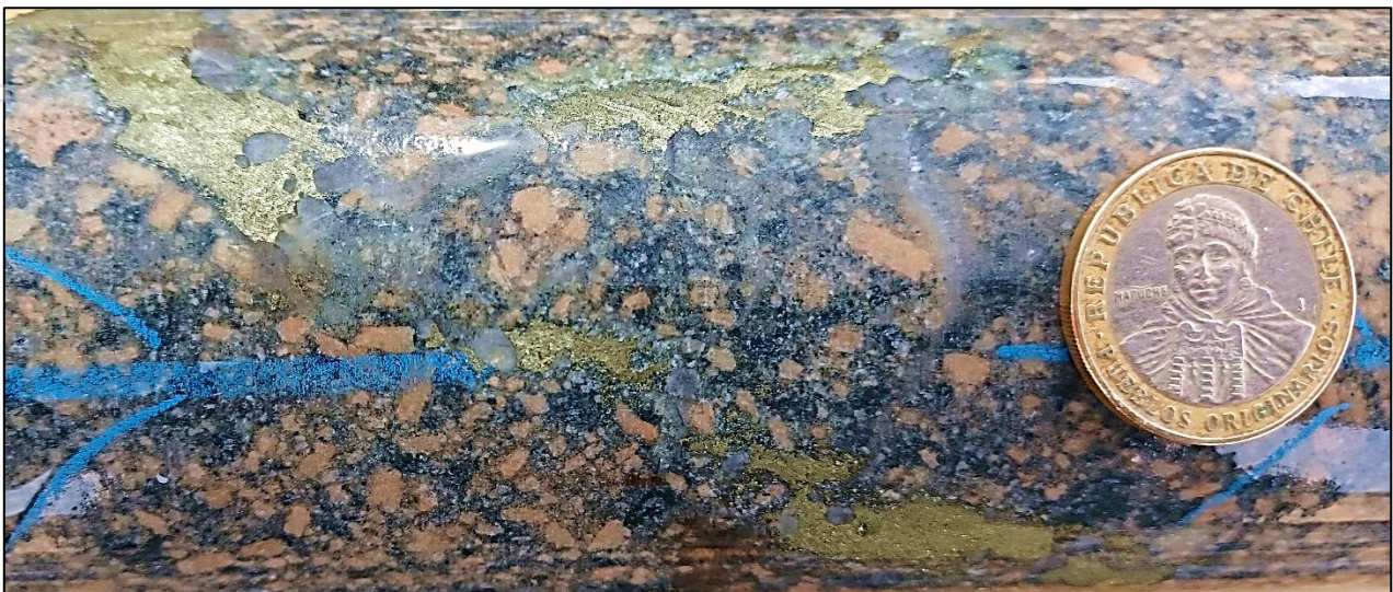
Figure 1: Example of high-grade copper mineralisation in hole CMLCD014, 1.74% CuEq (416m to 418m).
