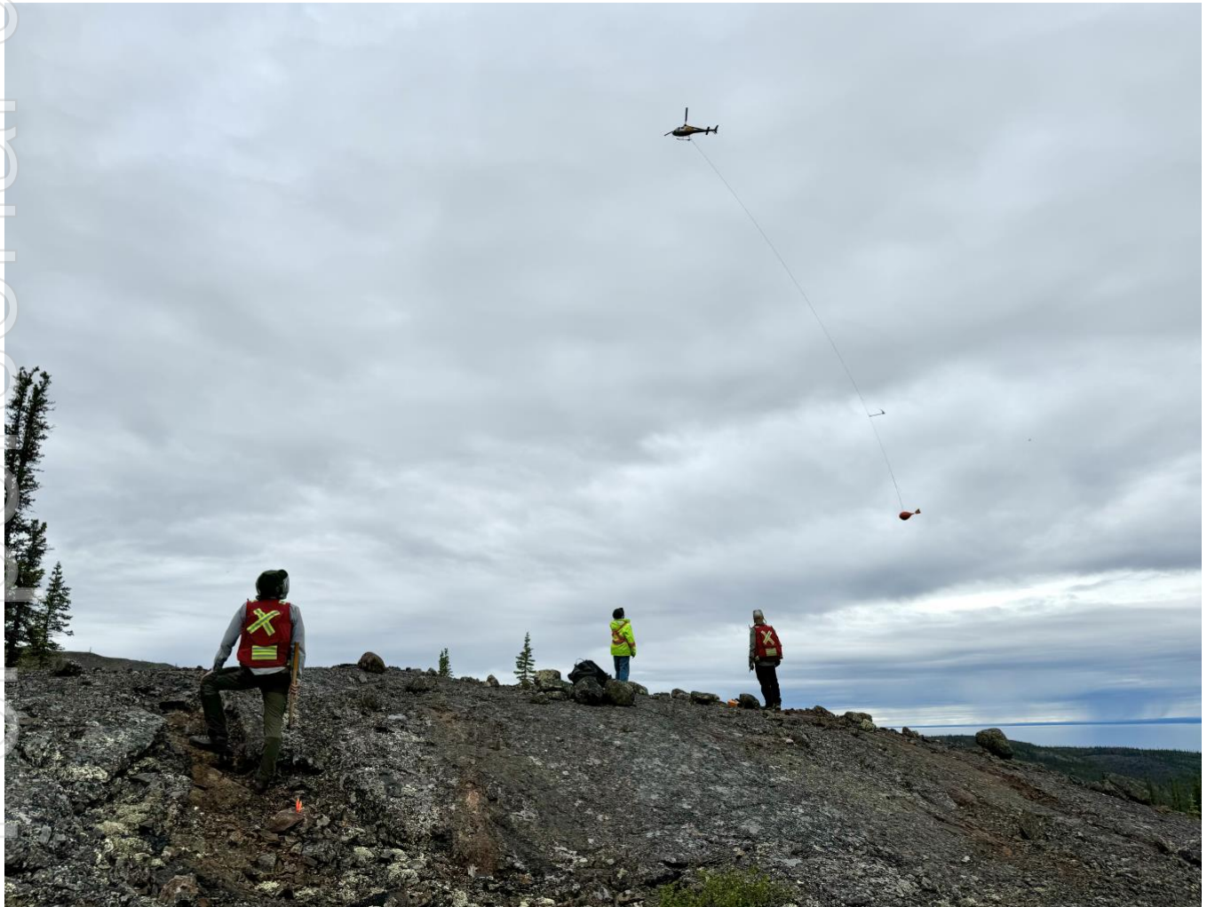
Figure 0 - Heli mounted MobileMT aerial surveys and field works underway at Great Bear Lake
