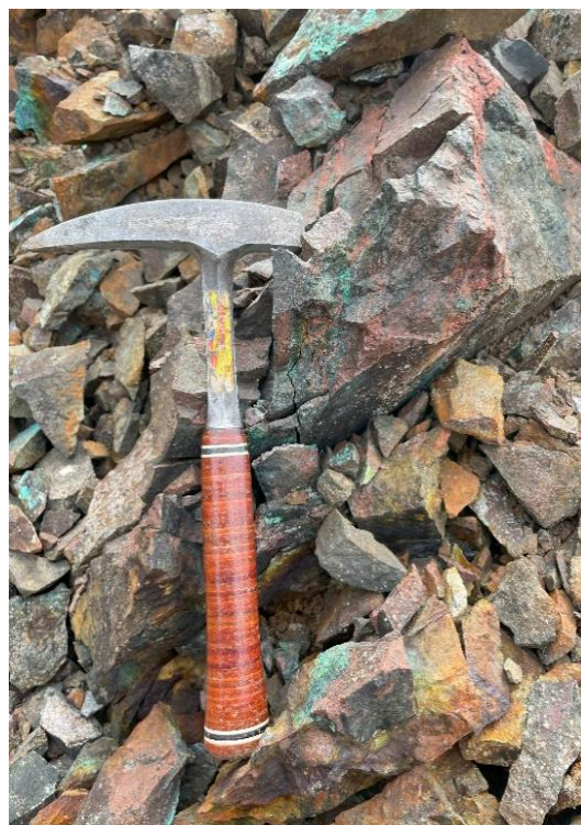
Figure 9 - Example of visually observed bornite-chalcopyrite cemented breccia (left) and strong brick red potassic alteration with observed chalcopyrite-malachite veining from the western extent of the Glacier IOCG target.
