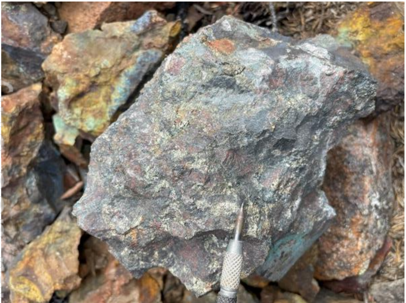
Figure 8 - Example of visually observed chalcopyrite cemented breccia from the western extent of the Glacier IOCG target. Clasts are composed of brick-red k-feldspar altered andesite.
