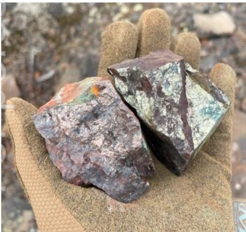
Figure 9 - Example of visually observed bornite-chalcopyrite cemented breccia (left) and strong brick red potassic alteration with observed chalcopyrite-malachite veining from the western extent of the Glacier IOCG target.
