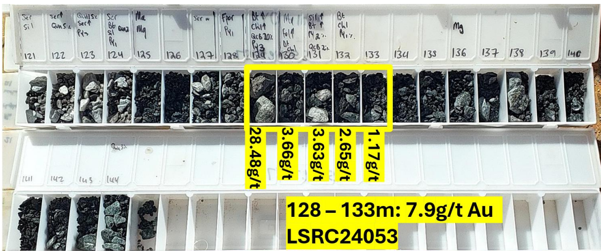
Figure 7 – Chip tray showing significant intercept at Pericles in LSRC24053 (5m at 7.9 g/t Au from 128m).
