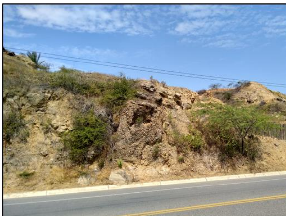
Ccoarse conglomerates in channels, followed by medium to coarse grained sandstones with conglomerate channels. Canoas Sector:
