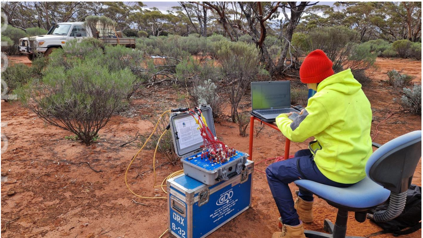
Figure 1. Collecting IP data at Miramar's 8-Mile target.
