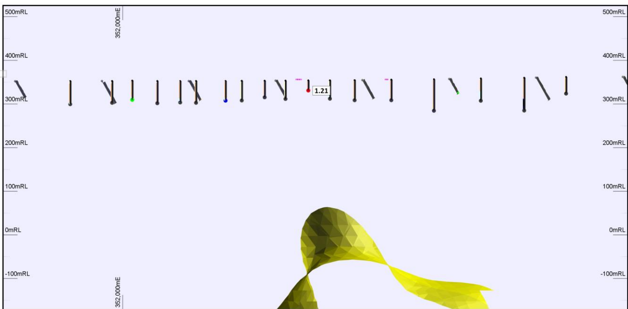
Figure 8. Cross section showing IP anomaly (yellow shape) beneath GJAC288 (1.21g/t Au at EOH).
