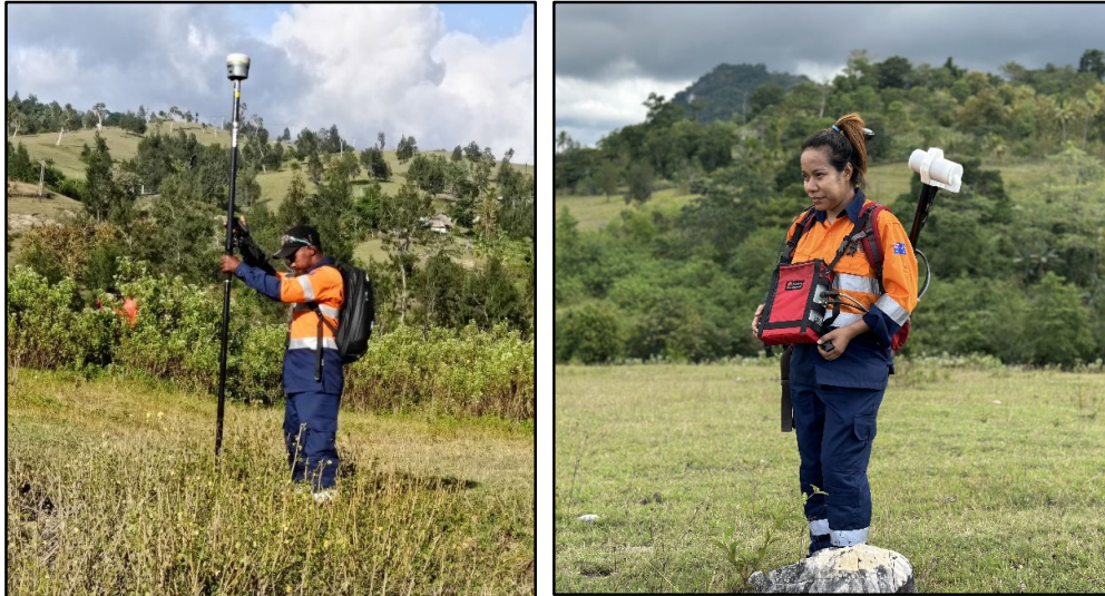
Figure 4a-b - Setting out the survey lines with DGPS and commencing ground magnetometer surveys. Beacon and its technical consultants are committed to the training and capacity building of local technical staff
