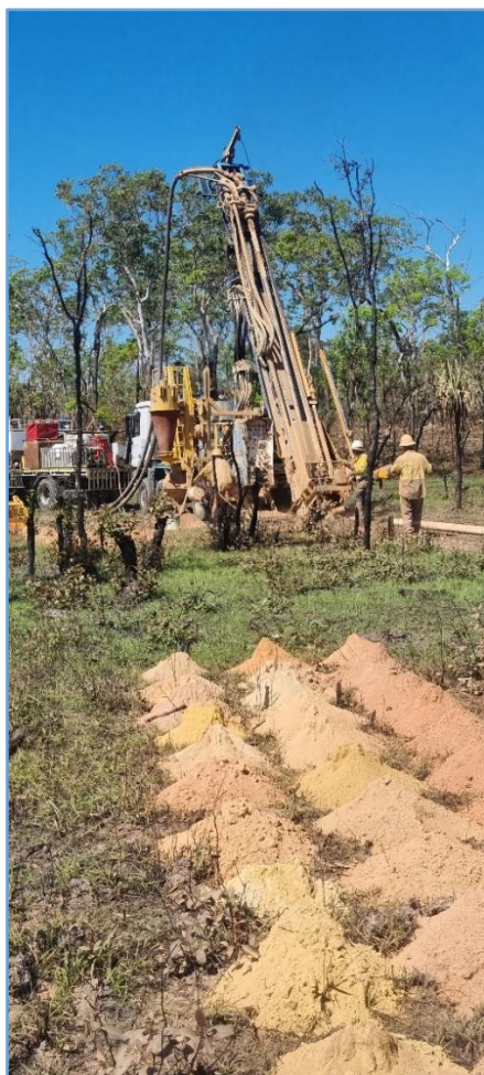
Figure 1: RAB drilling in the field at EverGreen's EL 31774
