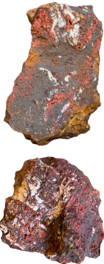
Figure 1: Ground truthing identified gossan. Figure 2 (Top): 1.91g/t Ag, 10.3ppm Sb, 14.7ppm As and 412ppm Zn, Figure 3 (Bottom): 2.6g/t Ag, 8.76ppm Sb, 30.7ppm As 303ppm Zn
