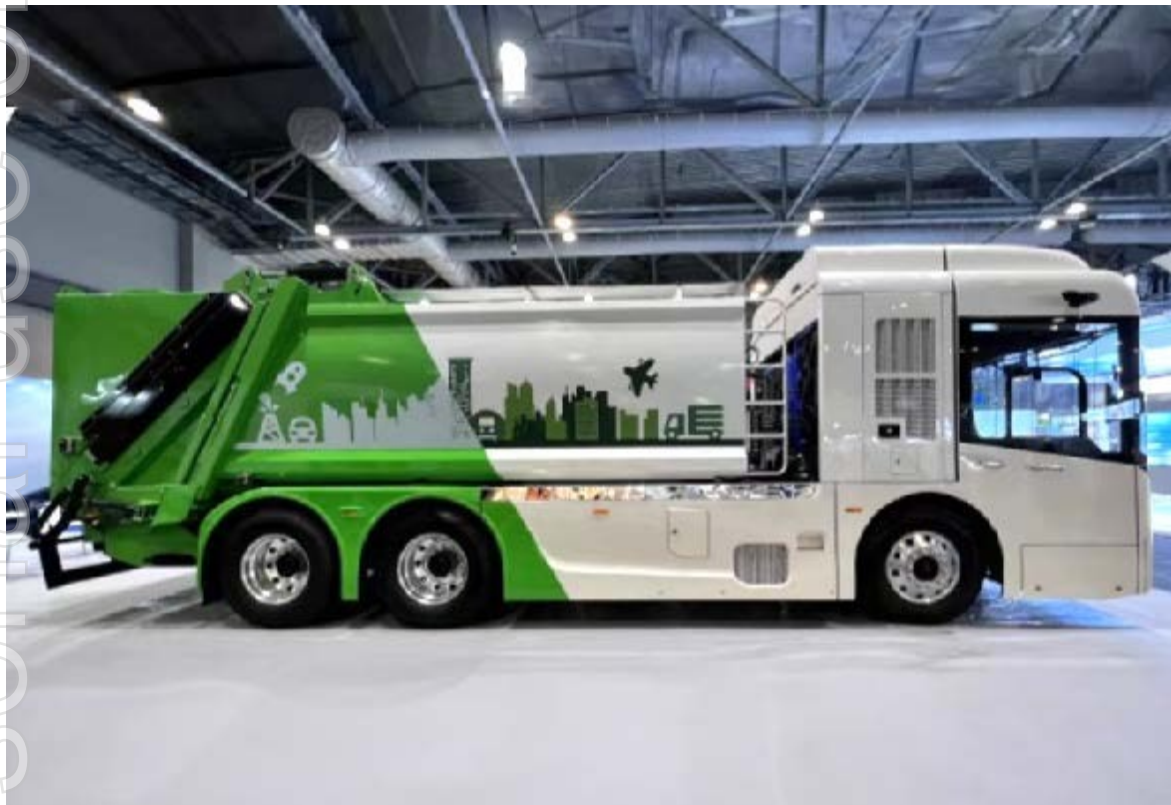
Picture of Hydrogen Fuel Cell Garbage Truck similar to the one that City of Newcastle has ordered
