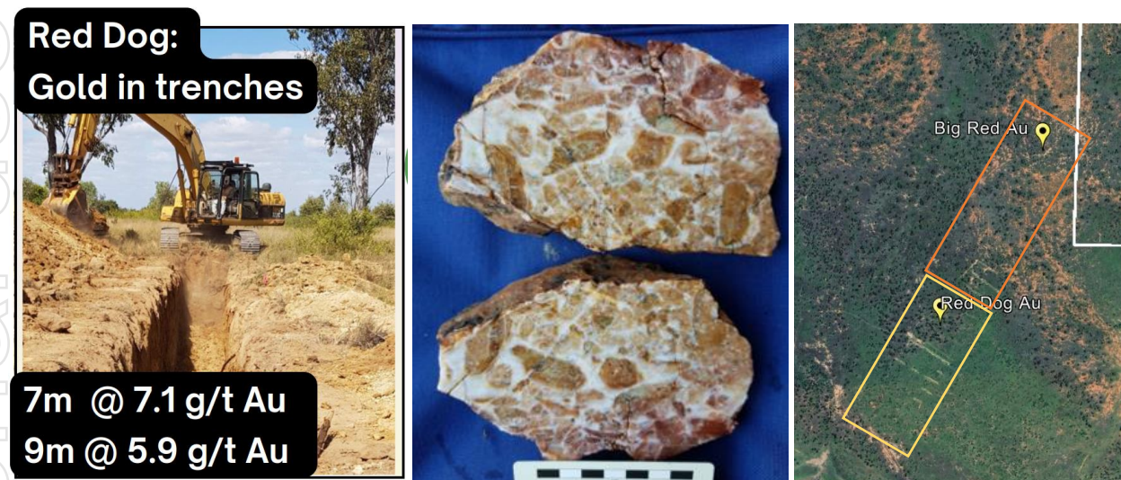
Figure 1: Big Red (Red Dog) Project –Past trenches; quartz breccias; area of past trenches (yellow rectangle) and planned extensions (orange rectangle)
