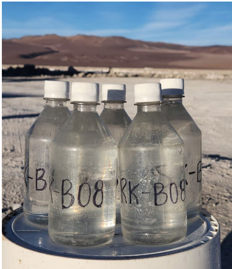
Figure 4 – Lithium Brine Samples collected from DDH-1 at the Rio Grande Sur Project.
