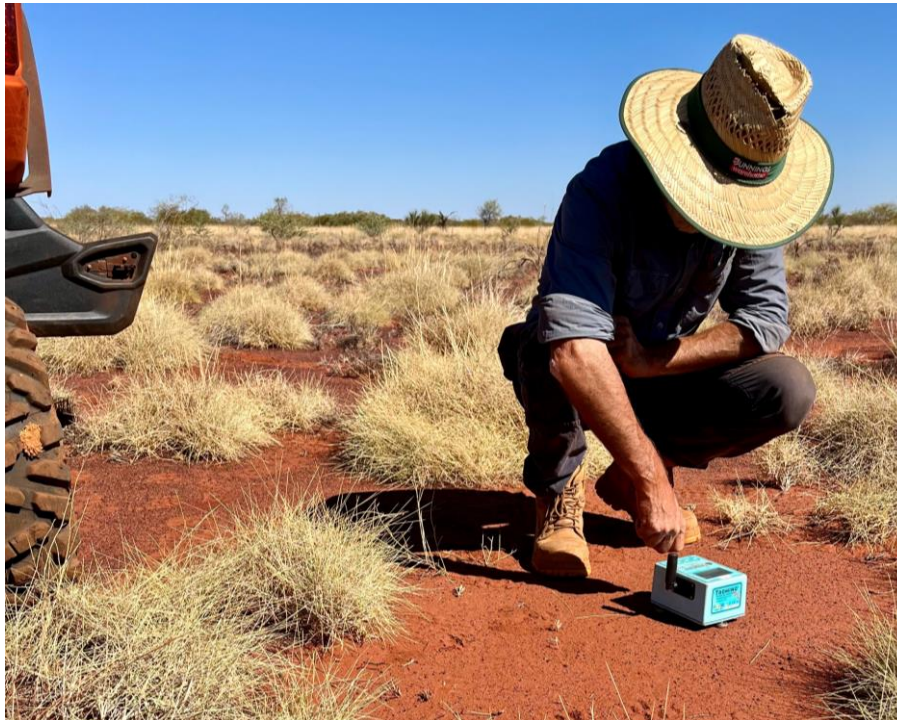
Figure 3. Miramar field staff collecting passive seismic data at the Whaleshark Project with a TROMINO seismometer.
