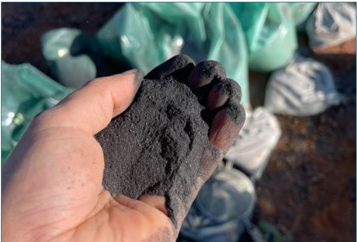
Figure 4: Typical black-coloured, heavy magmatic sulphide mineralisation at the Dante Reefs (HRC004).
