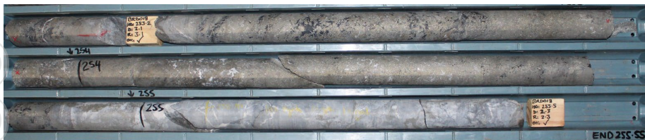
BRD018 , massive sulphide mineralisation (253.0-255.5m)
