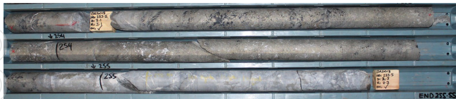
BRD018 , massive sulphide mineralisation (253.0-255.5m)
