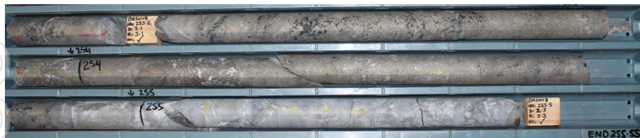
BRD018 , massive sulphide mineralisation (253.0-255.5m)
