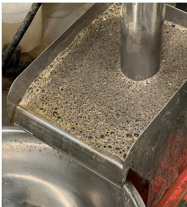
Figure 5: Niobium flotation during locked cycle
