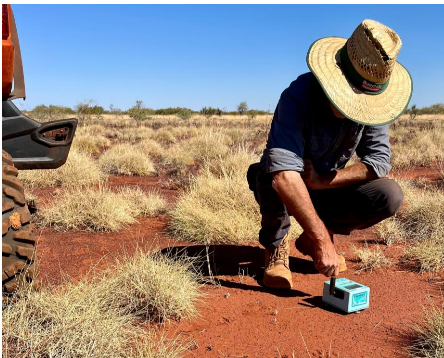
Figure 4. Miramar field staff collecting passive seismic data at the Whaleshark Project with a TROMINO seismometer.
