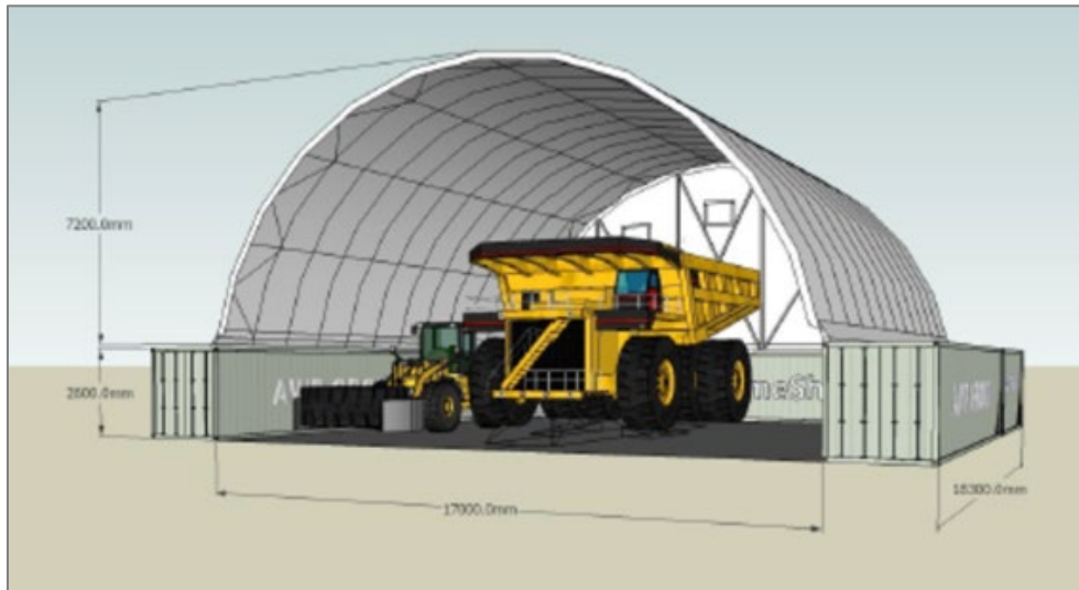
Figure 25: Example of Double-container height Haulpak workshop.
