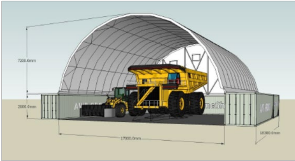
Figure 25: Example of Double-container height Haulpak workshop.
