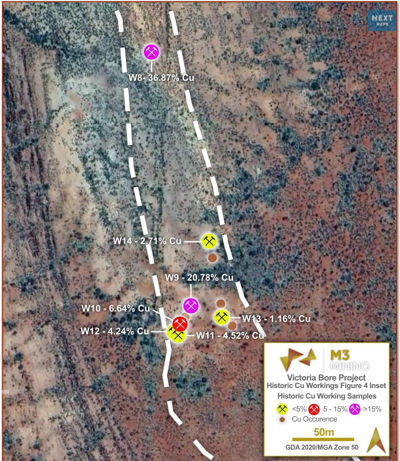
Figure 4 – Historic Copper Workings and pXRF Copper Soil Anomalism
