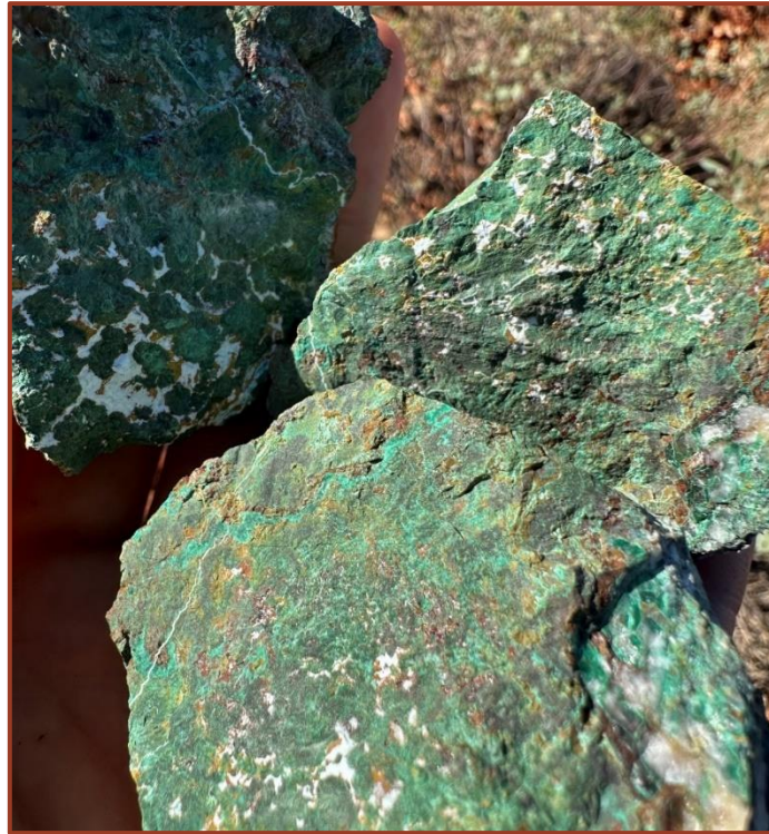
Figure 1 – Copper Oxide from Historic Working 8 (36.9% Cu)
