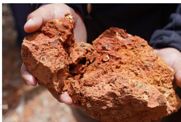
Photo 5 – Weathered Biotite- Granitoid from the Lourdes Areas (La Marigen). Notable Xenotime (black mineral) an indicator of REE mineralisation
