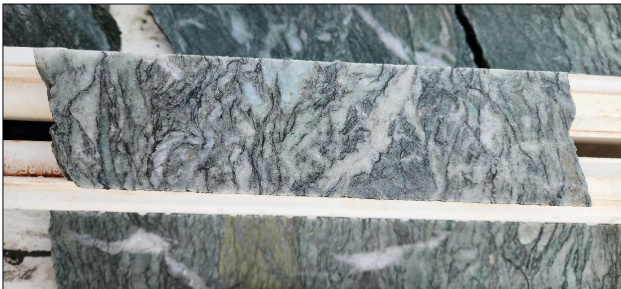
MLJDD019_148.4m_visceral texture in bleached, silicified ultramafic.
