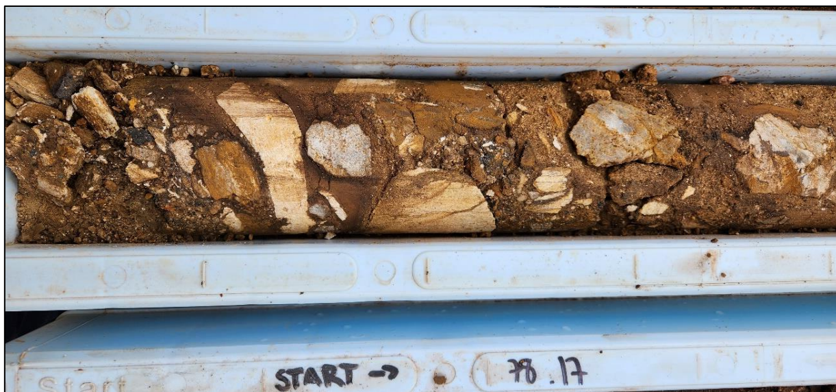
MLJDD020_178.0m_Polymictic Breccia with silica-pyrite clast
