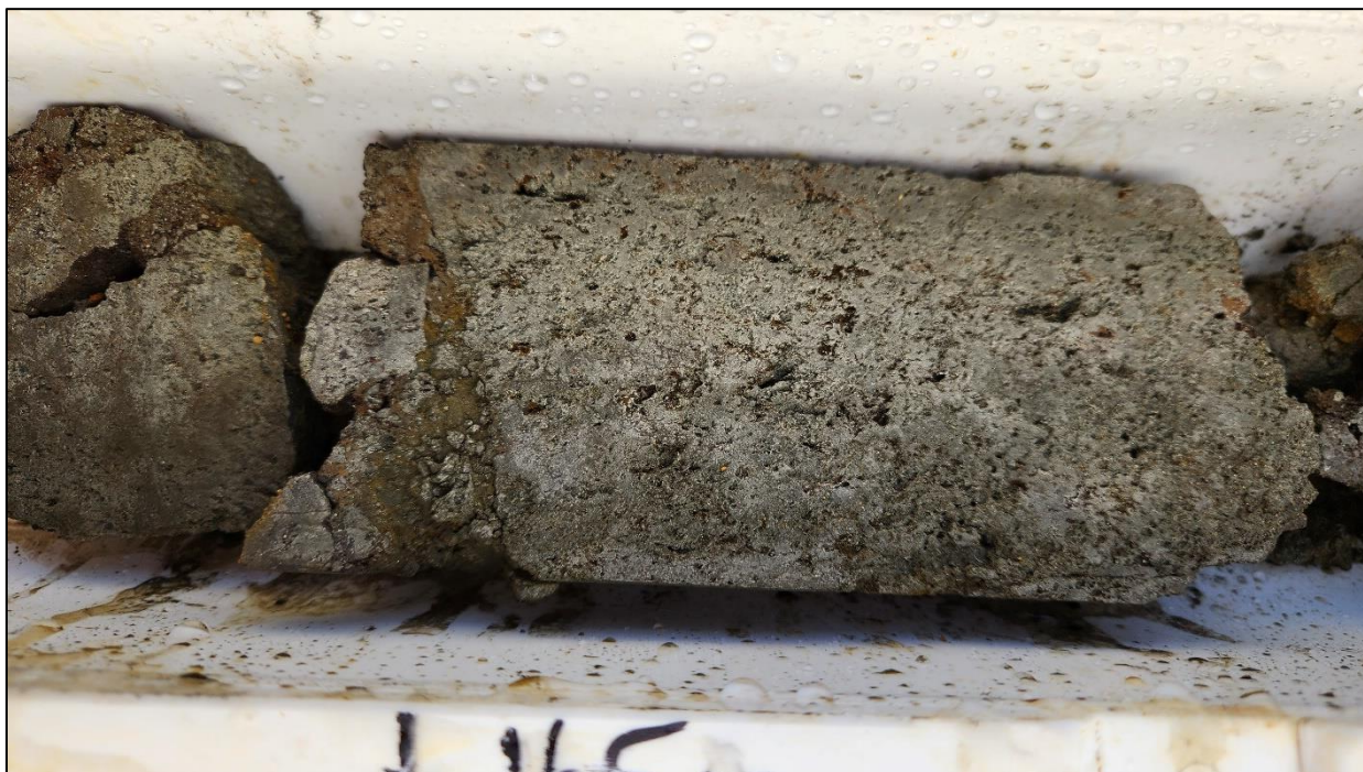
MLJDD018_164.5m_Massive pyrite in Breccia
