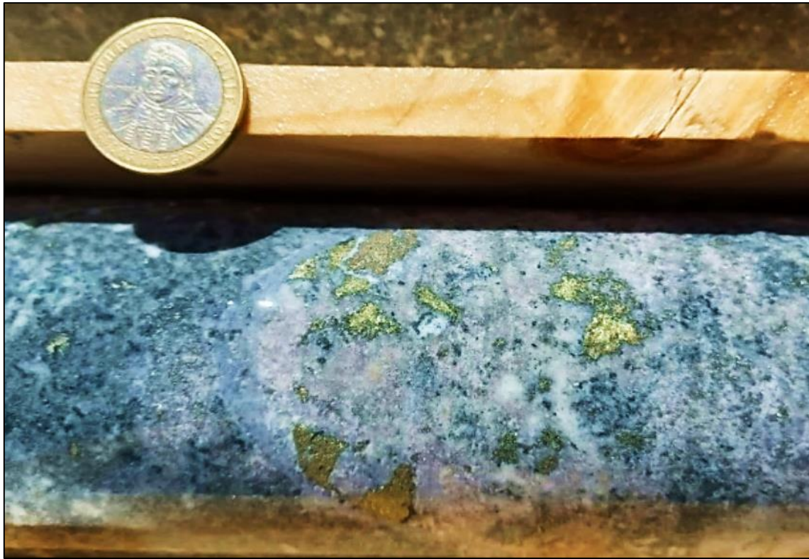
Figure 1: Example of high-grade copper mineralisation in hole CMLCD014, 2.71% CuEq (256m to 258m).
